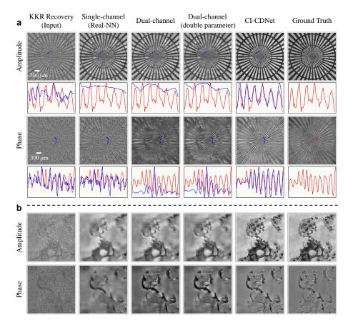
Figure S17: Comparison between CI-CDNet and dual-channel neural networks on experiment data (Kramers-Kronig-relations holography). (a) Results of Siemens star under 1 ms exposure time. (b) Results of papillary thyroid carcinoma slide under 1 ms exposure time.
