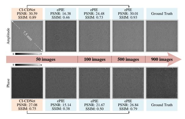
Figure S8: Quantitative results of lensless coded ptychography using different image numbers. The reconstruction results of CI-CDNet using 50 images are close to the results of ePIE using 500 images.
