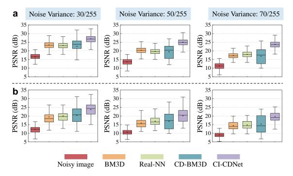
Figure S11: Quantitative results of 450 test dataset which added Gaussian noise (quantified by variance 30/255, 50/255 and 70/255). (a) and (b) are the results of amplitude and phase, respectively.
