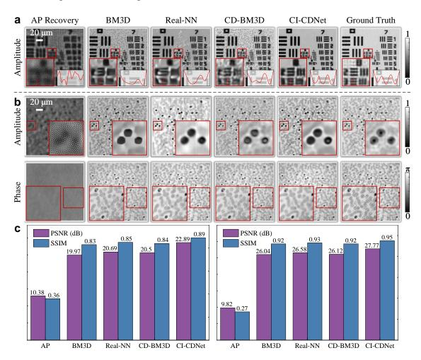
Figure S15: Additional results of Fourier ptychographic microscopy under 0.25 ms exposure time. (a) Amplitude results of the USAF resolution test chart. (b) Amplitude and phase results of blood smear. (c) Qualitative results of blood smear. The left histogram shows the PSNR and SSIM results of amplitude. The right histogram shows the PSNR and SSIM results of the phase.
