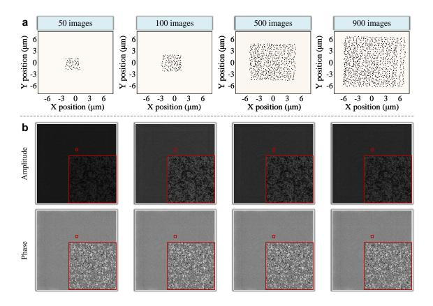
Figure S4: Principle of lensless coded ptychography (LCP). (a) Positions of the sample's shifts under different data volumes. (b) Reconstructed diffuser's profile under different data volumes.
