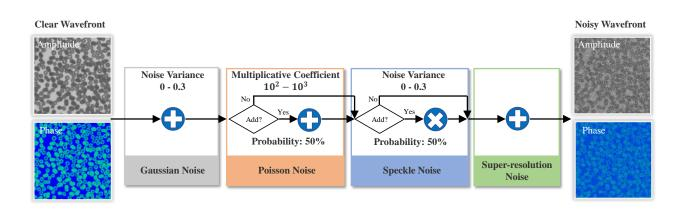
Figure S1: Noise model and parameters for constructing training data.
