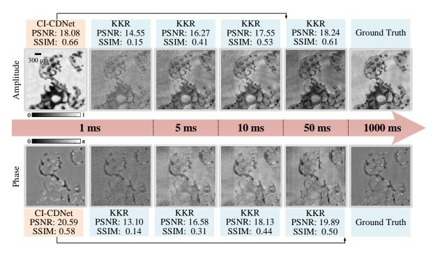
Figure S7: Quantitative results of Kramers-Kronig-relations holography under different exposure times. The reconstruction results of CI-CDNet under 1 ms exposure time are close to the results of KKR under 50 ms exposure time.
