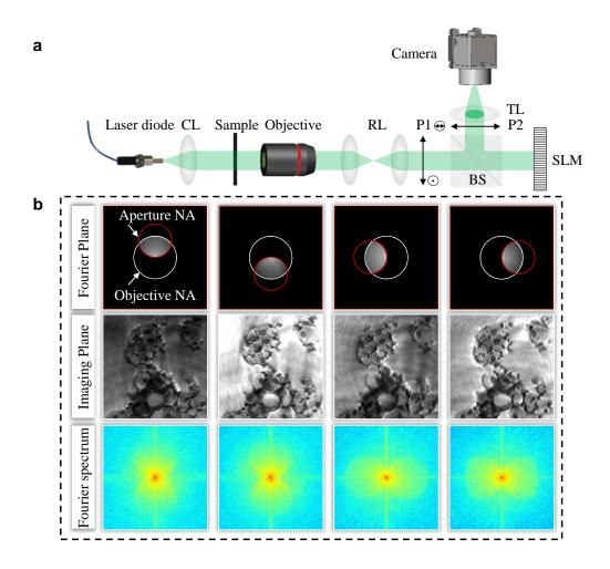
Figure S2: Principle of aperture modulation Kramers-Kronig-relations holography. (a) System diagram and setups. (b) Aperture modulation strategies (first line), intensity-only measurements corresponding to different subregions (second line) and Fourier spectrums of different measurements (third line).
