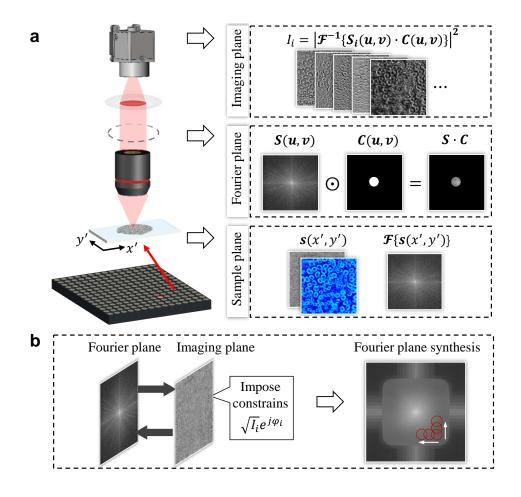
Figure S3: Principle of Fourier ptychographic microscopy (FPM). (a) Schematic diagram and setups. (b) FPM reconstruction principle.
